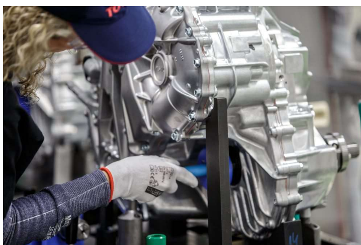
Transaxles fitted to the Corolla and C-HR hybrids
