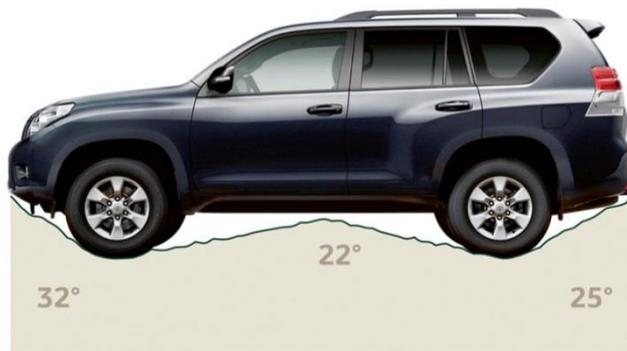
Ramp breakover angle (NB vehicle not 2014 model design)
