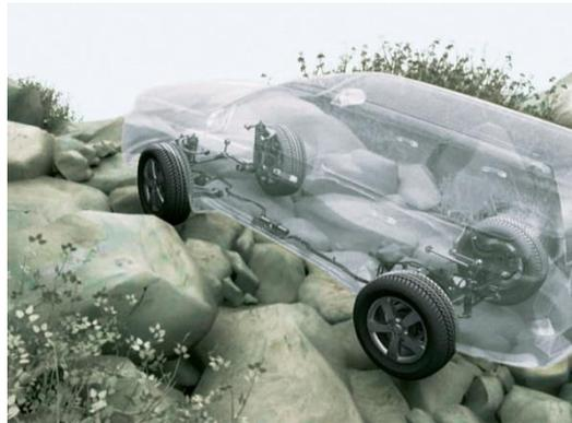
Drivers should choose an MTS mode on the basis of the amount of wheelspin encountered. For example, when excessive wheelspin prevents the vehicle from gaining enough traction, a more aggressive mode, closer to the Rock setting, should be selected. Conversely, when there is too little wheelspin to achieve the necessary traction, a less aggressive setting, closer to Mud and Sand is recommended.
