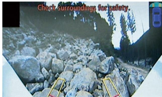
The side cameras let the driver view an image of the area around the left and right, front or rear tyres simultaneously, regardless of the vehicle's direction of travel.
