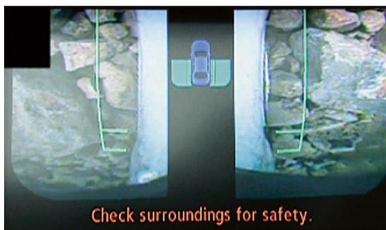
The monitor also displays comprehensive information relating to the front view, including the camera range and location of any obstacles detected by the clearance sonar. Steering-linked guidelines are shown, mapping the predicted path of the front tyres to help the driver avoid any hazards ahead. The inner and outer edges of the front tyre paths are shown in red (within 0.5m) and yellow (within 1.0m) to indicate the distance from the front of the vehicle.
