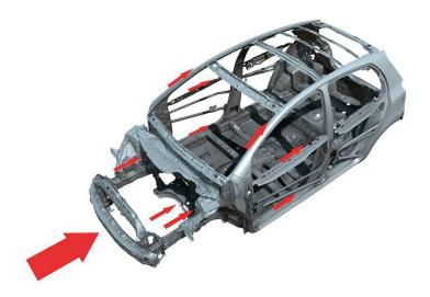
In the event of a head-on collision, impact energy is received by the front side members and transmitted to a complex under-body frame structure and to the upper body, through the A pillar and side bars in the front doors.
