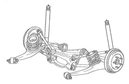
The trailing arms are made of single piece cast steel on which the wheel and coil spring carriers are integrated. The trailing arm is hollow to reduce weight. Angle and positioning of the trailing arm and bushing characteristics are designed to provide a toe-in effect upon braking. The attachment axle at the front of the trailing arm is angled toward the vehicle's axle.
