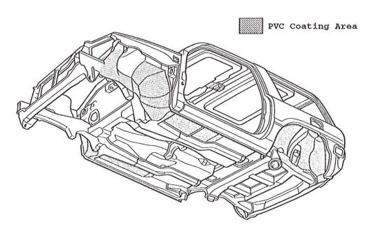
Anti-chipping paint and PVC primer are applied to the sill panels and front and rear wheel arches to protect them from flying stones. In addition, soft-chip primer is applied to the bonnet and front end panels.
