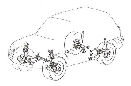
The long arms used on the RAV4's suspension ensure ideal camber variations and a generous amount of vertical suspension movement. If the suspension travel is short, the vehicle may bottom out on bumpy roads, or may have difficulty in keeping all four wheels in full contact with the road surface.
