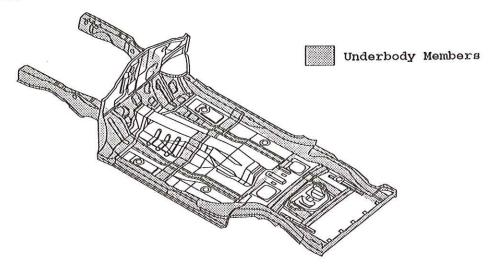
Rust-resistant performance is increased by using anticorrosion sheet steel and performing anti-corrosion treatment by applying wax, sealer, anti-chipping paint etc, to easily corroded parts such as the bonnet, doors, sill, panels etc.
