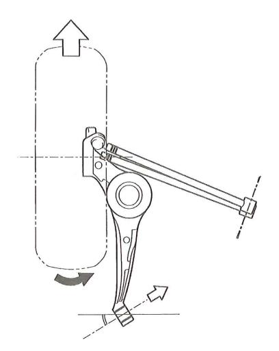
When the brakes are applied, the braking force pulls the wheel as well as the trailing arm backwards. The wheel that is attached directly onto the trailing arm effects compliance steer in the toe-in direction, ensure vehicle to stability during braking.
