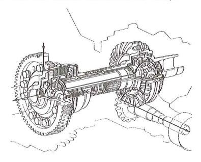
The automatic transaxle in the RAV4 is a 4-speed compact electronically controlled (ECT). The centre differential, front differential and transfer gears, whose function it is to transmit the power from the transaxle to the front drive shafts and the propeller shaft, are enclosed within the automatic transaxle case.
