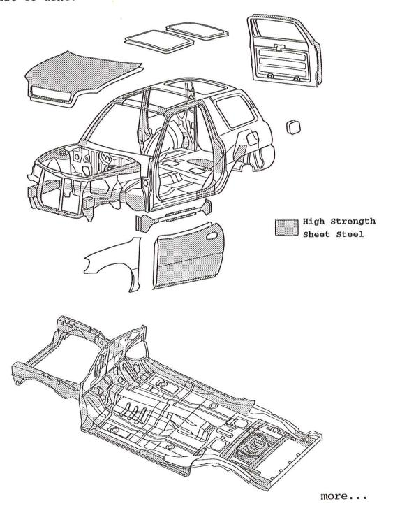
When an accident does occur, the CIAS (Crushable Impact Absorbing Structure) construction transfers the impact energy beneath the sturdy passenger cell, via the underbody structure. Side protection beams improve door rigidity, and are provided as standard.
