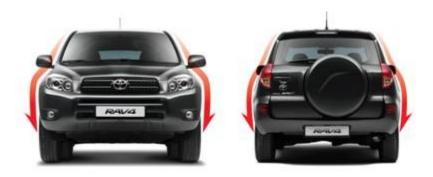
The vehicle is 145mm longer than the previous generation model at 4,395mm (4,315 for T180 without rear-mounted spare wheel) and has a significantly longer wheelbase (+70mm) and rear overhang. This allows passenger comfort to be greatly improved: cabin length is up by 85mm (to 1,820mm) and the couple distance between front and rear seats is greater by 55mm.
