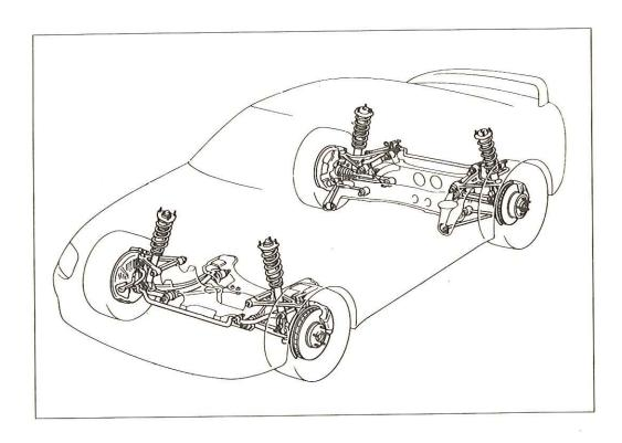
The redesigned chassis holds the road with new coil-over shock absorbers with hollowed front and rear anti-roll bars for high rigidity with reduced unsprung weight.
